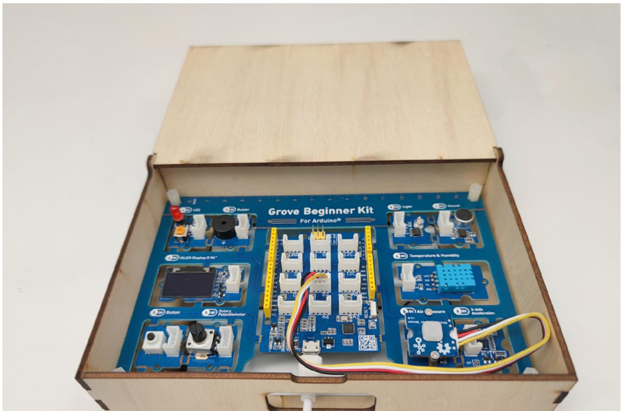
Then connect the additional module with Grove wires to Grove Beginner Kit pins:
