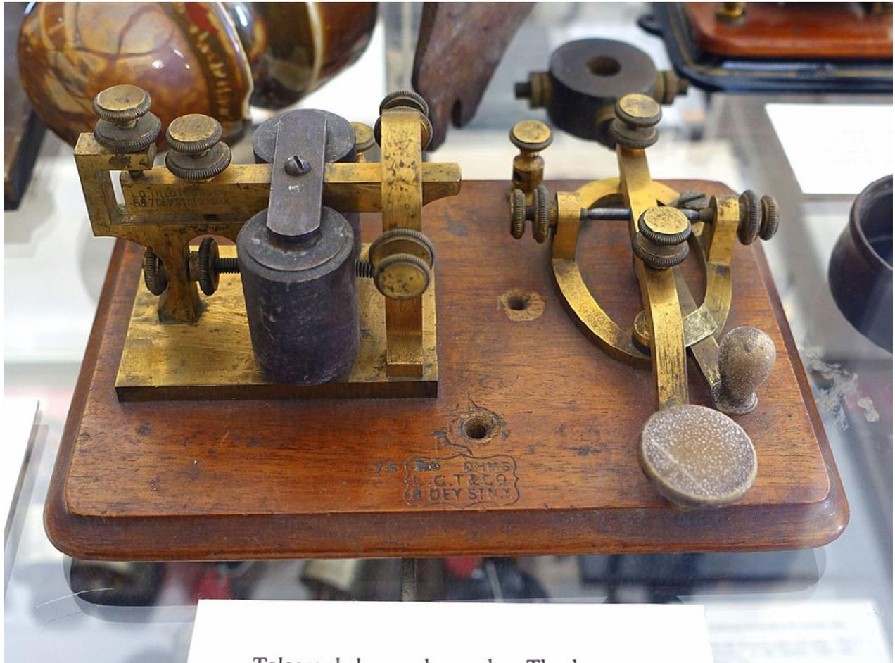
Telegraph key and sounder. The key was used to send Morse code.
