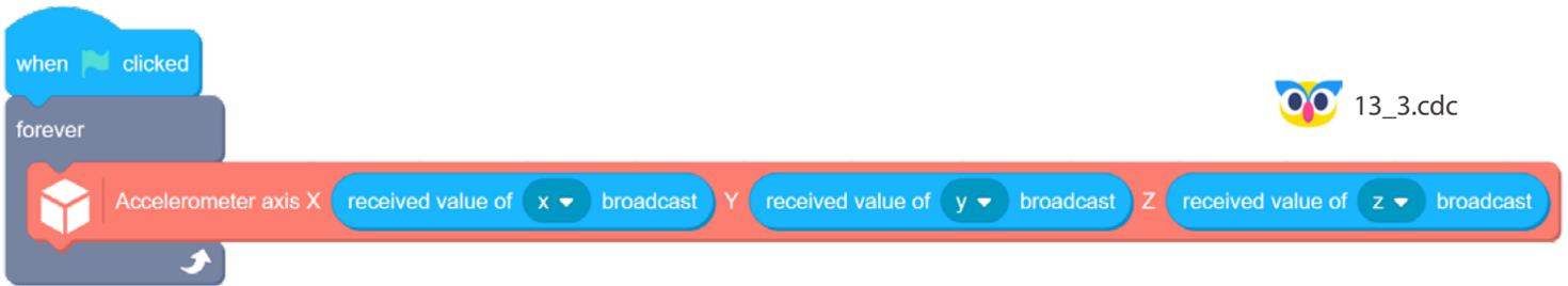
Connect to Arduino in Device mode as you usually do when use Serial monitor or Plotter. Then go to stage mode, press the flag button and click on **Open 3-Axis Accelerometer window** button in 3-Axis Accelerometer visualization category. The data flows from the sensor to Grove Zero Beginner kit mainboard and then to computer, where it is visualized in the browser window. Pretty cool isn't it?
